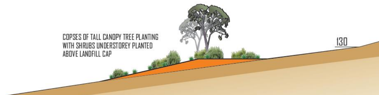
Figure 8-4 Typical planting on topsoil mounds on top of landfill cap
